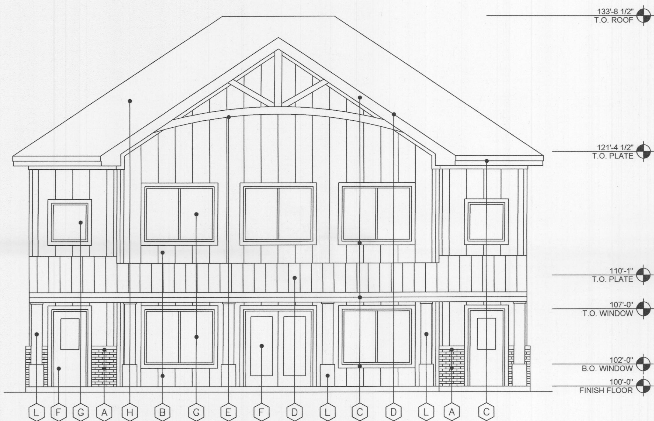
3 WEST ELEVATION - MASONRY: 6% SCALE: 3/16" = 1'-0"
