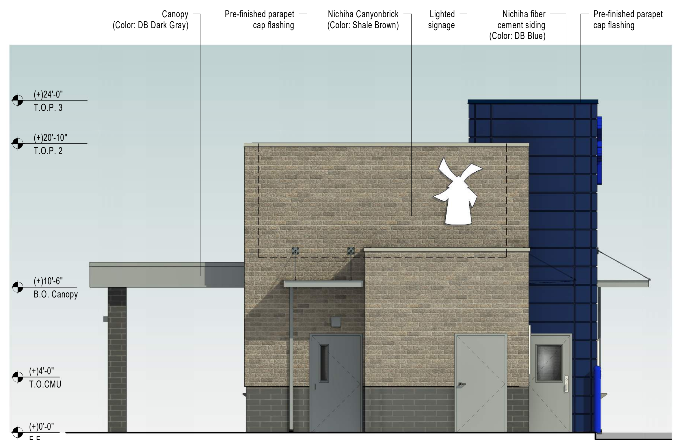
West Elevation - (Rear Elevation) 1/4" = 1'-0"
