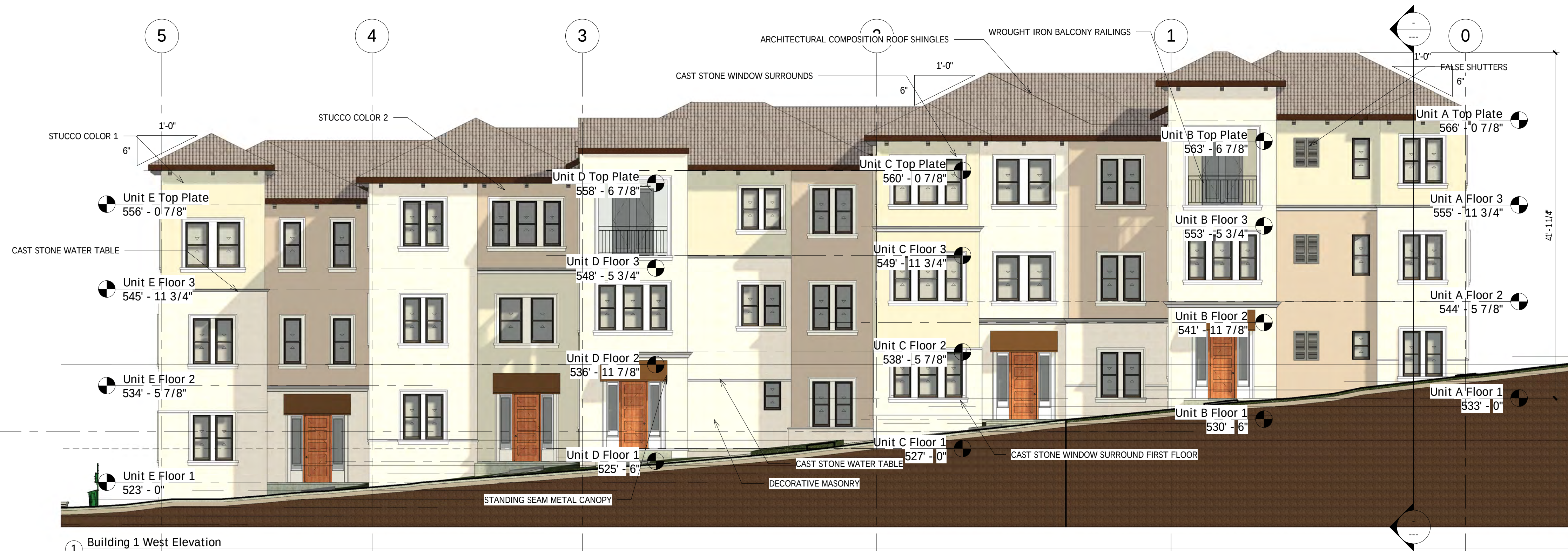
① Building 1 West Elevation 1/8" = 1'-0"
